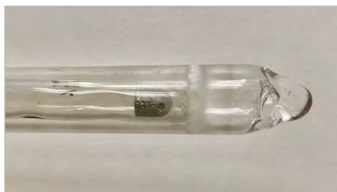
Figure 1: (Left) Diffractogram of the antimony Telluride. La phase Sb 2 Te 3 corresponds to all peaks. (Right) Crystal produced after a full Brdgmán growth
