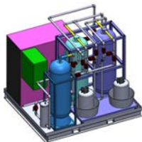
First visuals of the water treatment SKID
