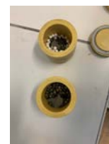
Sediments in grinding pots. Dry and melt with acetic acid.
