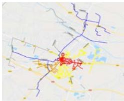
BRAM map showing leakage rates in the network according to colour (red: high leakage rates) (before installation of the pressure stabiliser)
