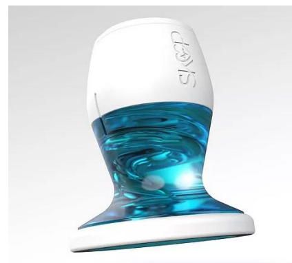
Representation of The Skop - 3D-printed connected stethoscope
