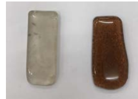
glass from commercial silica on the left and glass from rice husk on the right
