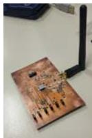
Picture of the finished Eval-board
