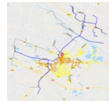
BRAM map showing leakage rates in the network according to colour (red: high leakage rates) (after installation of the pressure stabiliser)
