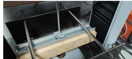
First pull out test on the bench
