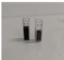
Photographs of carbon nanotube dispersions (two different surfactants); the mass proportions are identical in both cases, so we can see macroscopically that the BS disperses the nanotubes better
