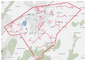
Plan of the at-risk pipes on the Salindres drinking water distribution network
