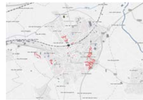
Plan of the pipes at risk on the drinking water distribution network of the commune of Lunel (Canopée software).
