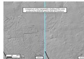
Comparison map of topographic shadings of the raster produced by LiDAR HD and the RGE ALTI database
