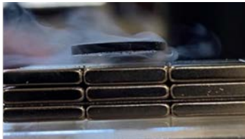
levitating superconducting YBCO pellet
