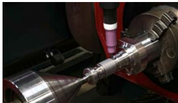
Production and welding of a "bellows/ring" qualification assembly.
